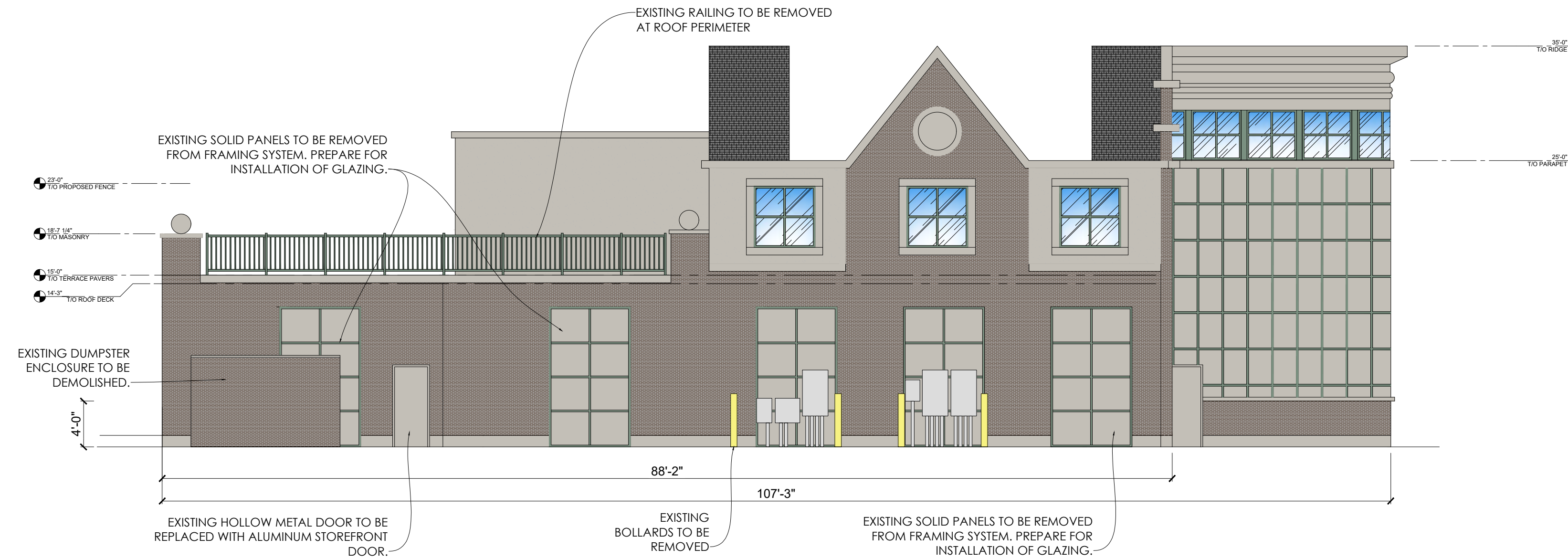
Exist/Demo West Elevation
