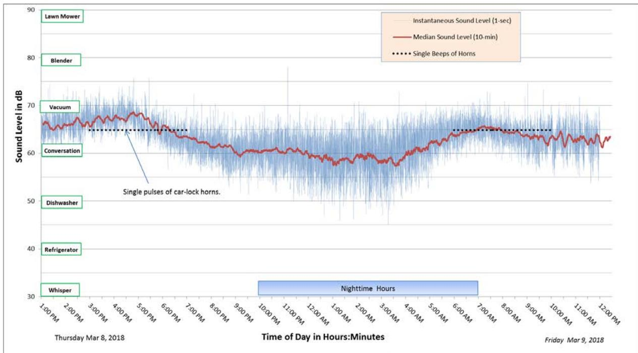
**Figure 3 – Ambient sound levels recorded over a nominal 24-hour period near the residential area just east of the proposed garage.**
